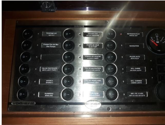
**Figure 4 DC Panel, Refrigerator ON**
