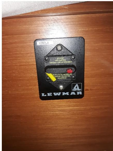
**Figure 3 Windlass Circuit Breaker (Open/OFF)**
