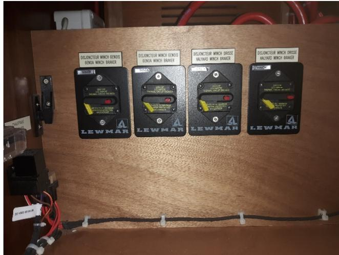
**Figure 2 Winch Circuit Breakers (Open/OFF)**
